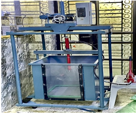
Fig. 5 A steel box with dimensions of 600 mm × 600 mm × 600 mm used in the study.
