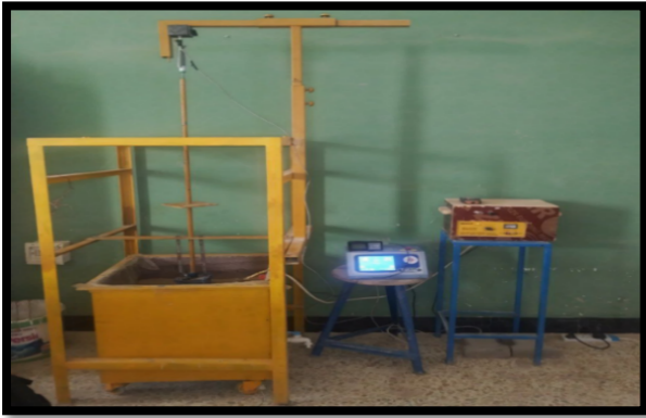
Fig 8 The container with specimen, the steel footing model and the fixed LVDT
