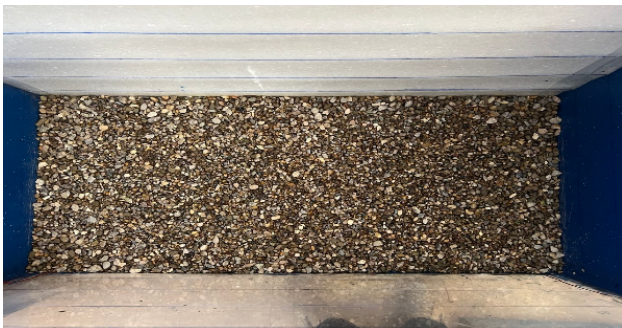
Fig. 5 Gravel layer at bottom of container
