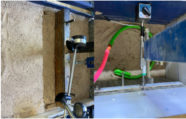
Fig. 1. Cyclic load test following the preparation of the sheet pile wall and soil
