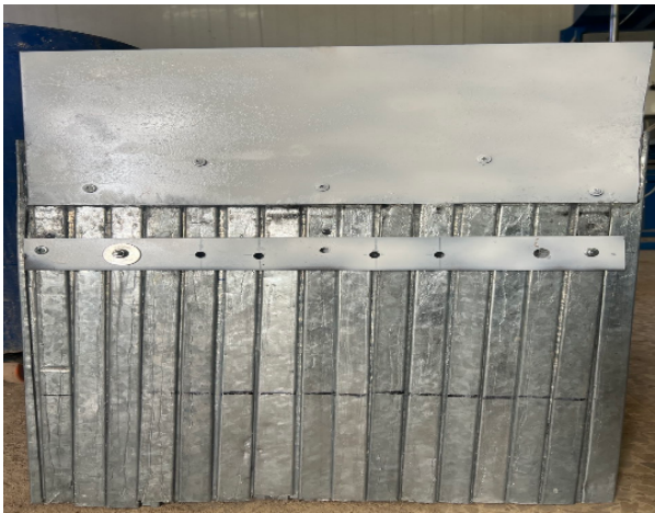
Fig. 1 Sheet pile wall with plate
