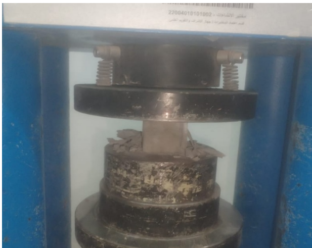
Fig. 6 Sample after compressive strength test
