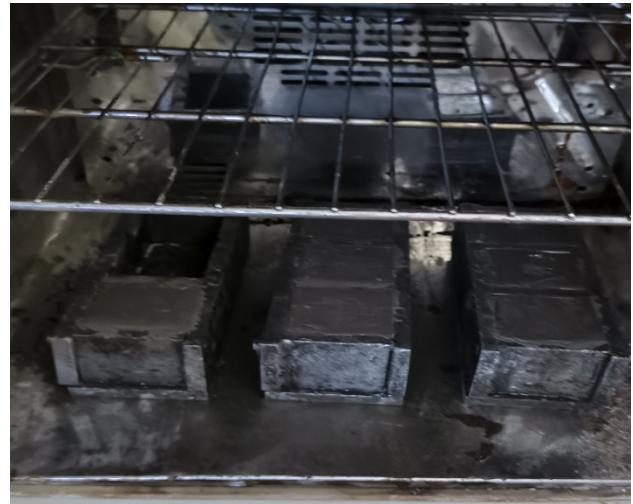
Fig. 3 Samples under heat curing at 90°C
