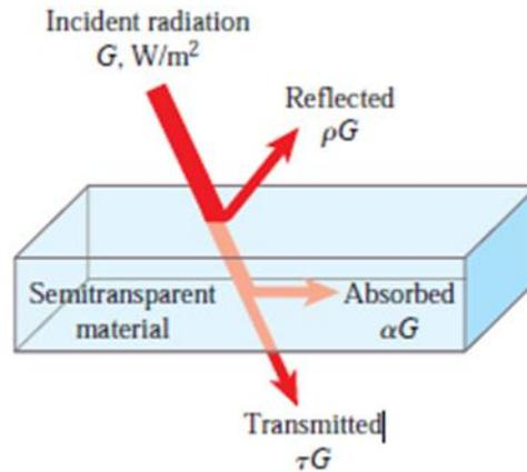
Fig. 2 Heat through collector by semitransparent material [5].
