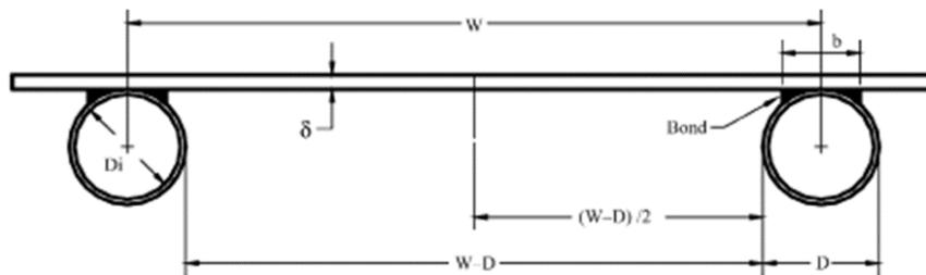
Fig. 3: Tubes arrangement of Flat-plate solar collector [11]
