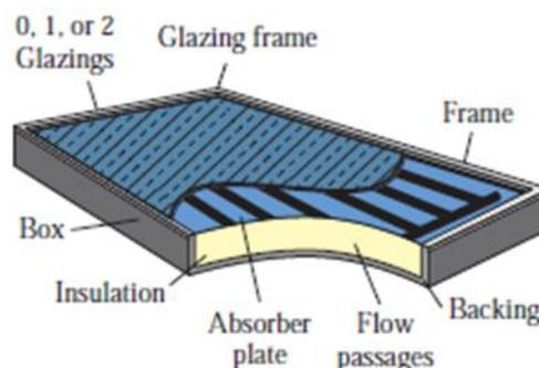
Fig. 1 Components of Flat plate solar collector [4].
