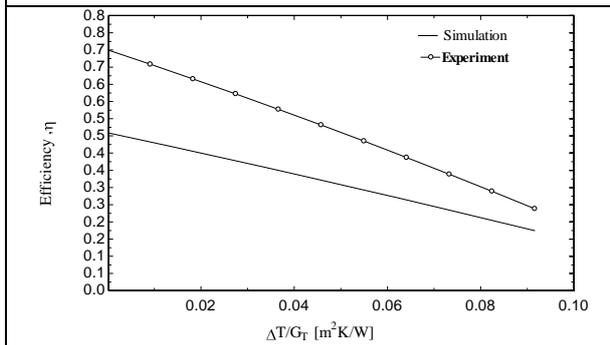
Figure 7. Efficiency of Collector during 2<sup>nd</sup> condition
