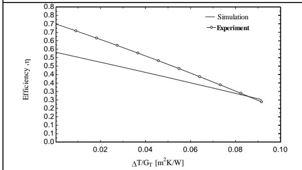
Figure 8. Efficiency of Collector during 3<sup>rd</sup> condition
