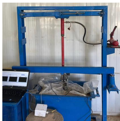
A) Experimental setup of the hydraulic jack and container
