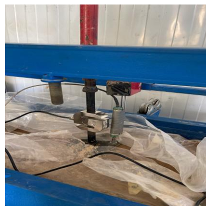
B) Details of the loading cell system with LVDT
