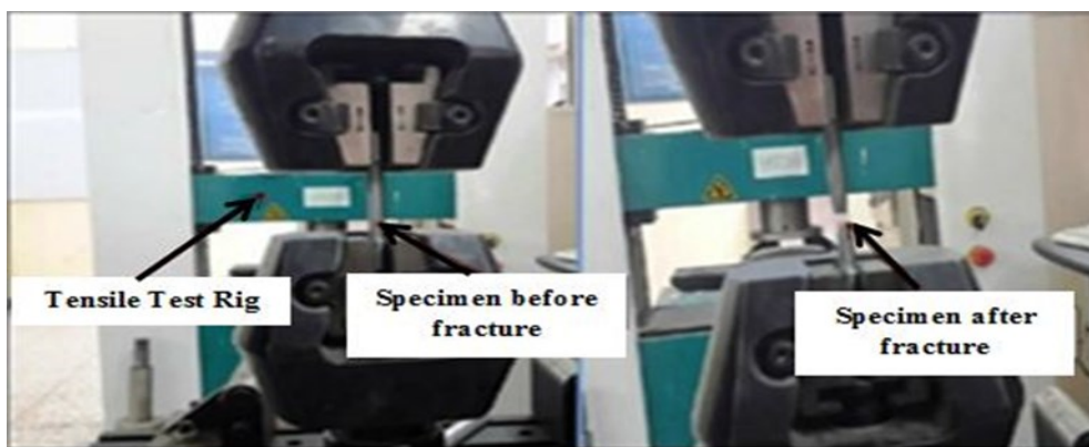
Fig. 2 The tensile test sample is produced as a circular form according to the ASTM
