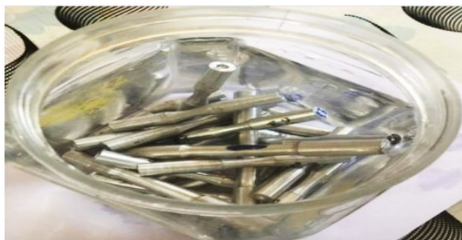
Fig. 4 Corrosion container for 3.5wt%, NaCl solution
