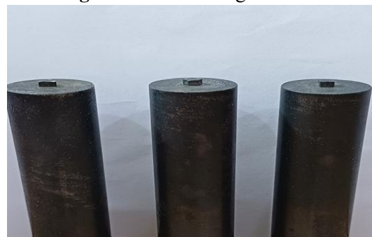
Fig. 2 Tool pin profiles of FSW: Triangle, Hexagonal, Square (the shoulder diameter: 18mm, pin length: 1.5 mm, and tilt angle 1°)
