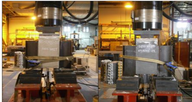
Fig 11: Push out test system at fire (a) ordinary concrete (b) carbon nanotube concrete [16]
