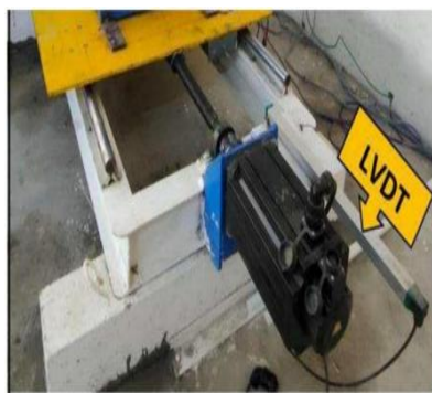
(A) The displacement sensors (LVDT) (with a range of 500 mm).
