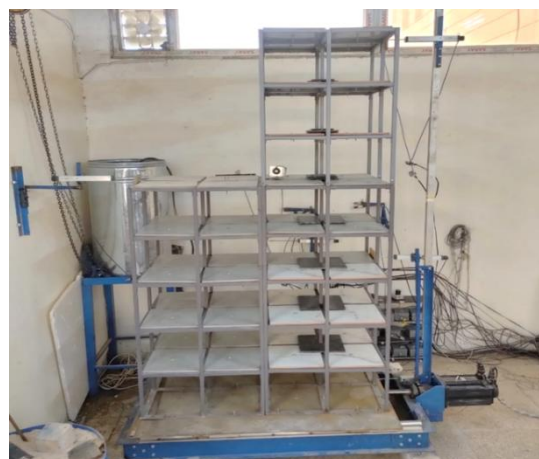
Fig. 3 Two steel models, five-story and eight-story, on a shaking table at zero-gap.
